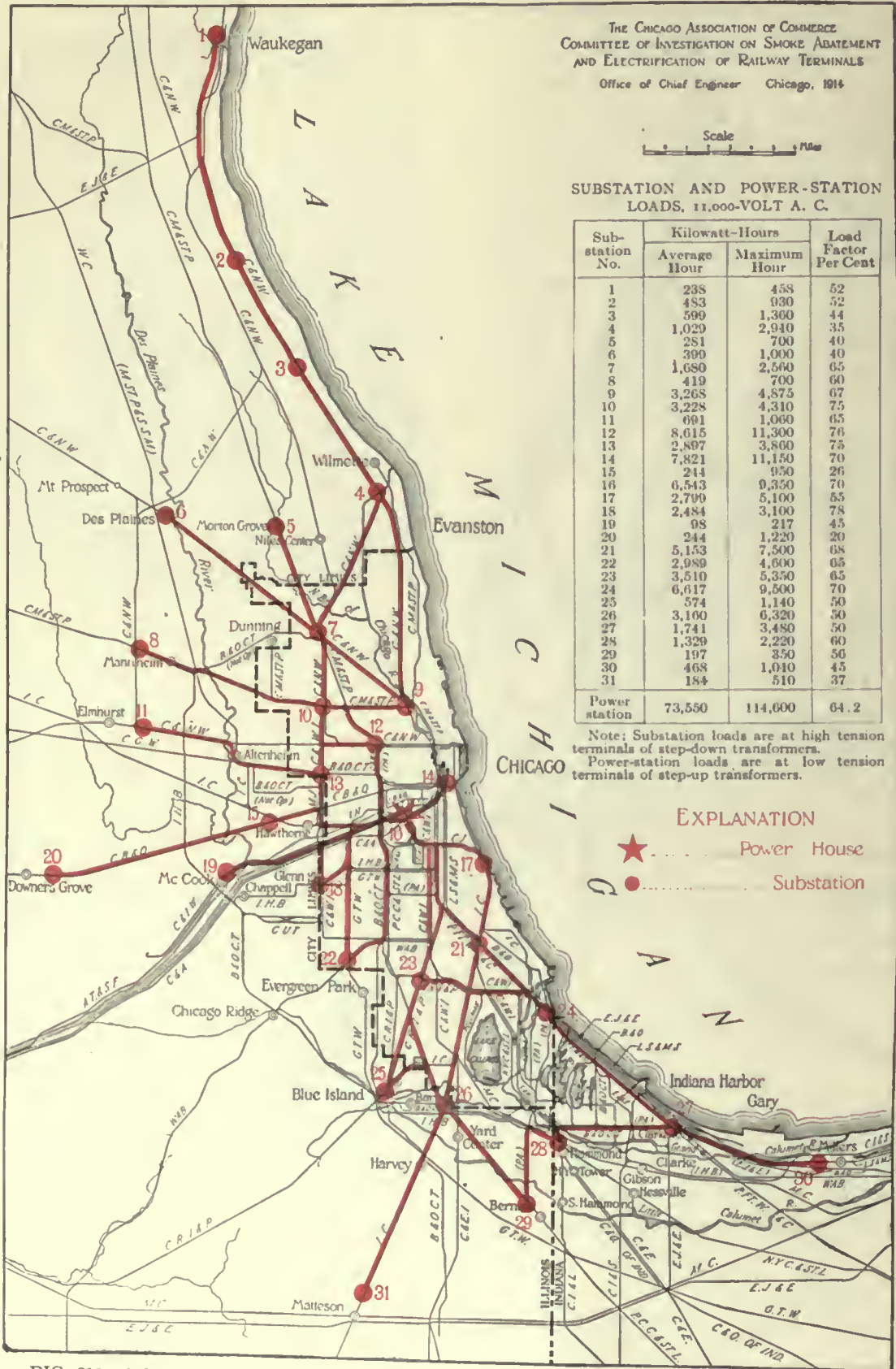
FIG. 610. LOCATIONS OF POWER STATION AND SUBSTATIONS FOR THE 11,000-VOLT A. C. SYSTEM
